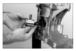
Position the piston with the arrow pointing towards the exhaust port.
